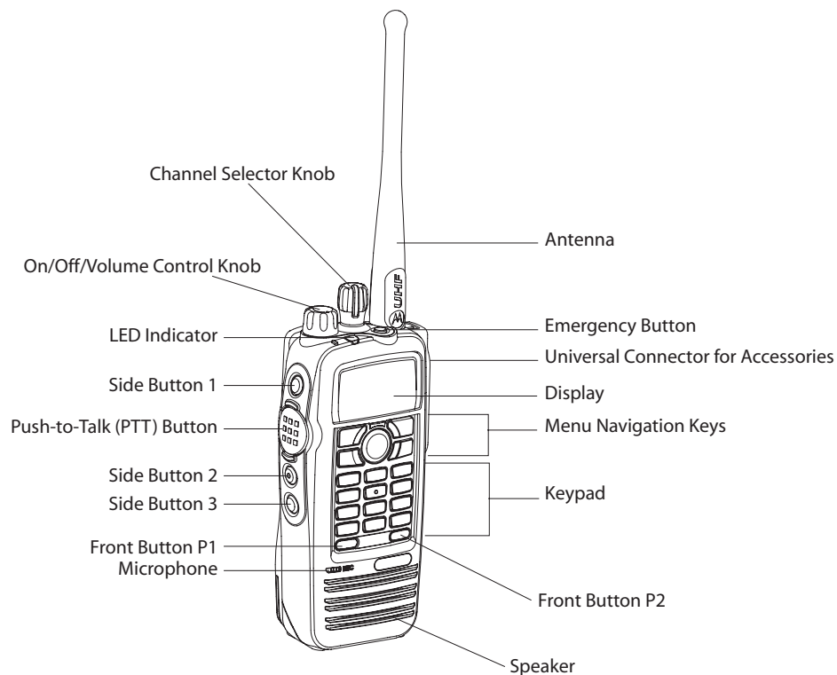
Figure 3-2 MOTOTRBO Portable (Display Model)
