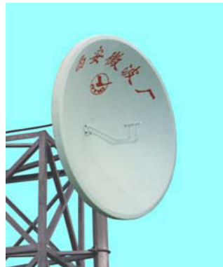
Figure2.5 Cassegrain antenna
