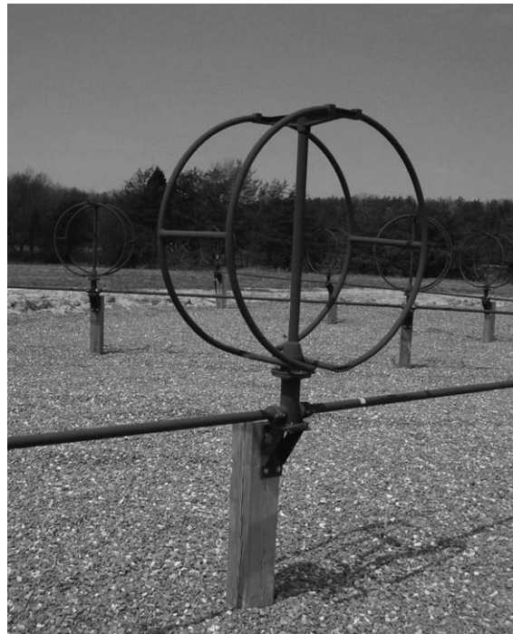
Figure 8.7: The Hermes Active Loop, post-mounted, with air-speed transmission lines to make it part of an array. Photo courtesy of US Antenna Products LLC, Frederick, MD, U.S., which is the current manufacturer.
