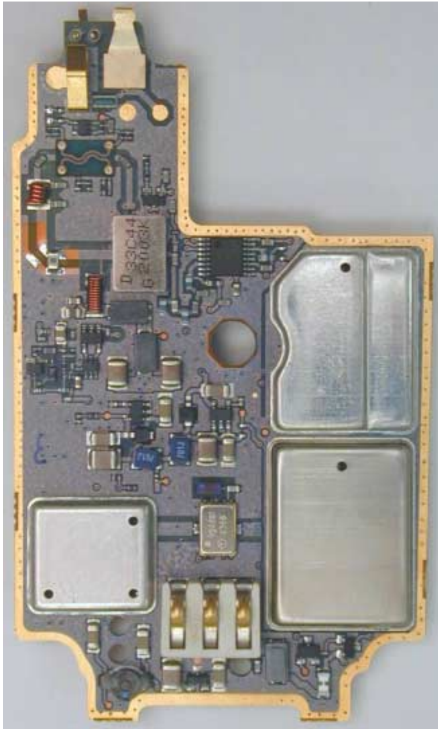
RF board with Shields (Bottom)
