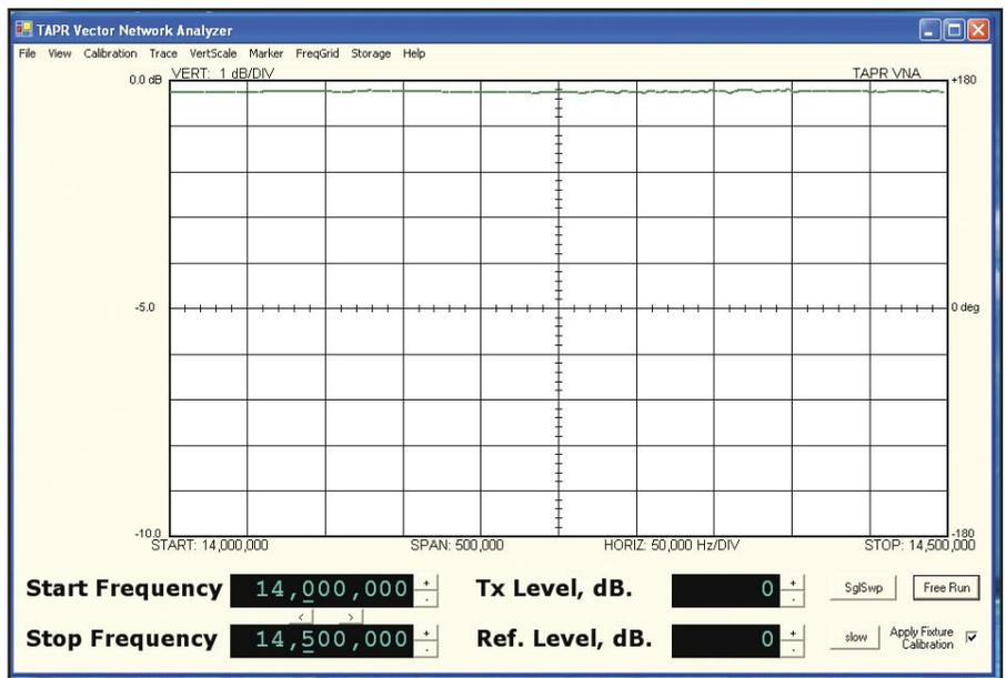
Figure 2 — Here's a closer look at insertion loss within the pass band of the filter. The model 6000 VNA is now measuring the response from 14 to 14.5 MHz, and vertical divisions are 1 dB.
