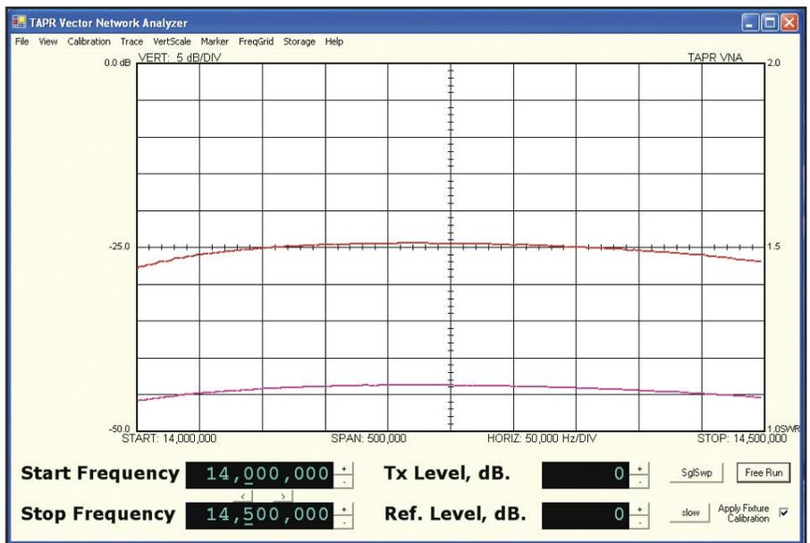
Figure 3 — Here's a look at the bandpass filter's input reflection coefficient. The model 6000 VNA is again looking at 14 to 14.5 MHz, and vertical divisions are 5 dB. The red trace near the center shows return loss, while the pink trace near the bottom shows SWR.
