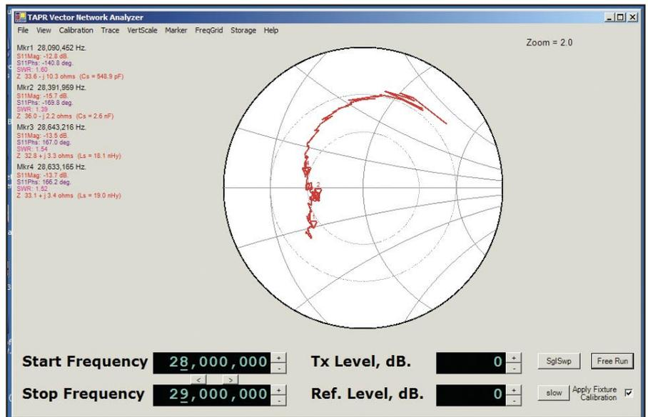
**Figure 4 — The polar display mode shows test results in a Smith Chart format. The model 6000 VNA is testing a 10 meter beam over the frequency range of 28 to 29 MHz. There are four frequency markers and the values for impedance and SWR are shown to the left of the plot.**
