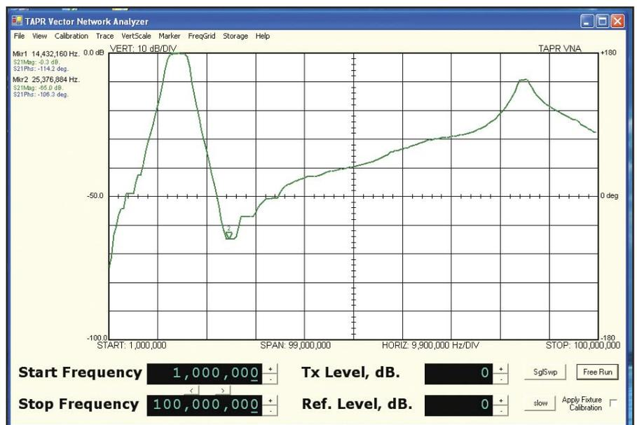
Figure 1 — Response of a 20 meter bandpass filter over the range of 1 to 100 MHz as measured with the Ten-Tec/TAPR model 6000 VNA. Vertical divisions are 10 dB. Insertion loss is 0.3 dB at 14.4 MHz, and stop band attenuation is 65 dB at 25 MHz (in the notch near the second harmonic frequency).
