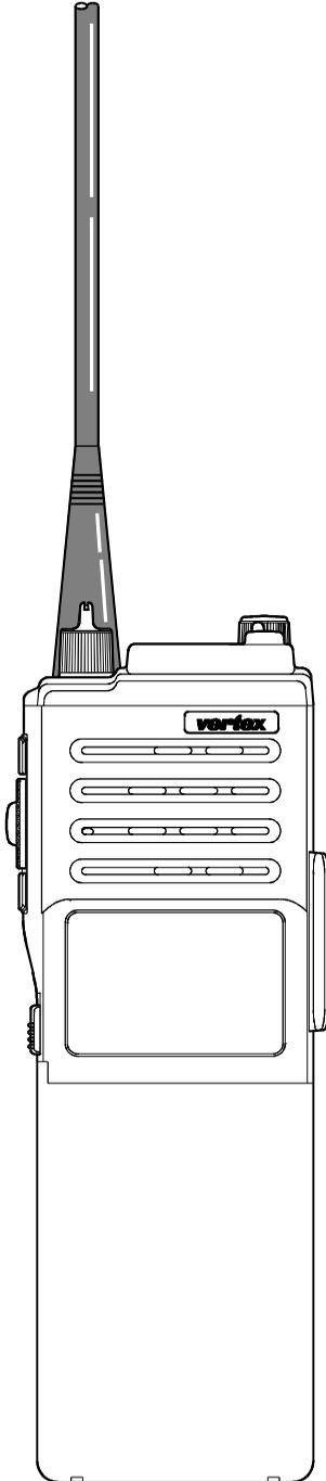
The VX-520U is a frequency-synthesized, microprocessor-controlled FM hand-held portable transceiver providing up to five watts of power output on up to 32 channels in the UHF Land Mobile Band. Designed specifically for commercial and professional applications, the VX-520U is housed in high-strength die-cast aluminum alloy, sealed to MIL-810 C, D & E intrinsically safe (I/S) and weather-tight specifications.
