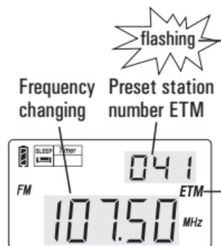
**Notes:** While operating ETM to search for stations, a few stations might be missed if there is interference in the surrounding. In this case, you can simply key-in the frequency, then press the [ETM] button to manually store it into ETM memory.
