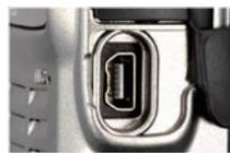
A USB connector is also located on the side of the radio. The optional microphone with camera (MH-85A11U) may be connected to this port.
