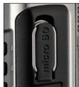
The micro SD card slot is provided on the side of the radio. The GPS logger records the location and track information of the moving station in the memory record inside the radio, the picture image data and other useful information data is stored on the micro SD card.
